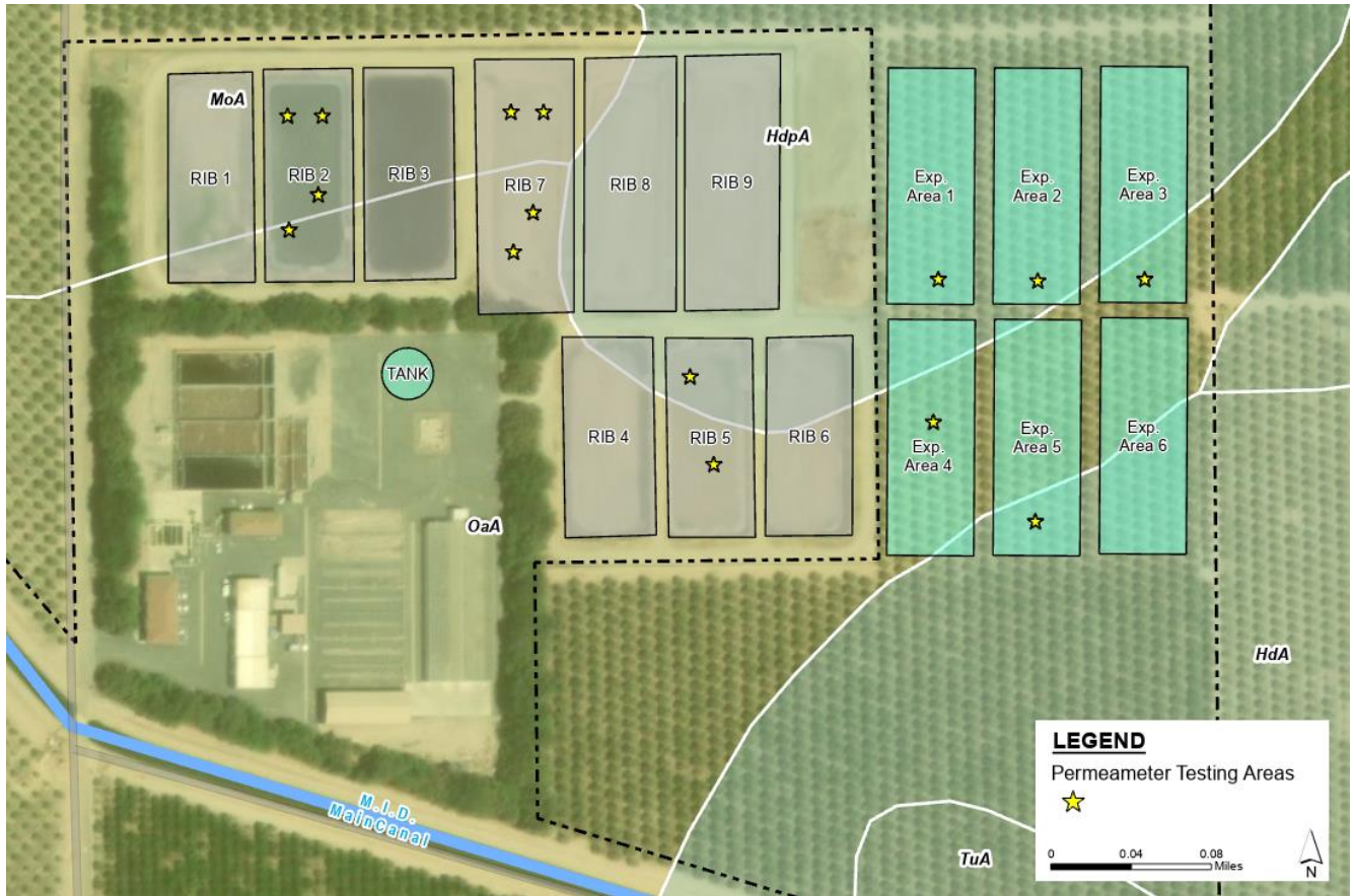
Figure 3 Permeameter Testing Locations
