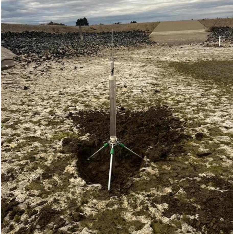
Figure 4 Example Surface Permeability Testing of RIB 5 by Guelph Permeameter December 2023
